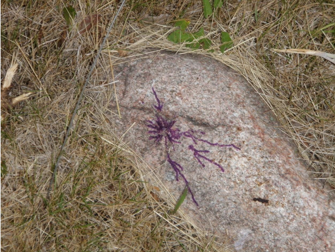
Figure 5 - GPS control point, marked on flat rock on island.
